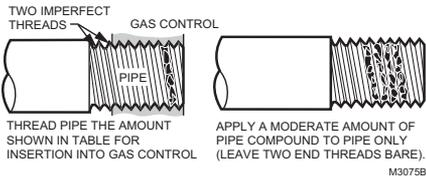
Fig. 2. Use moderate amount of pipe compound.
