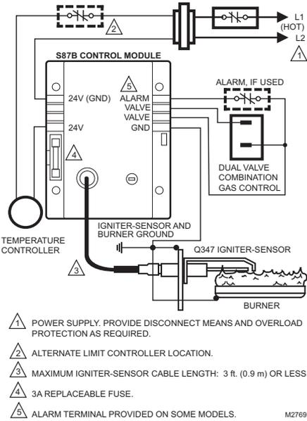
**Fig. 5. Typical wiring connections for 24 volt control in S87 Direct Ignition System.**
